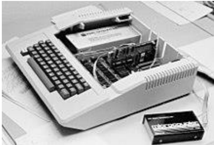
Figure 2. Apple II with an external modem, designed primarily by Wozniak
